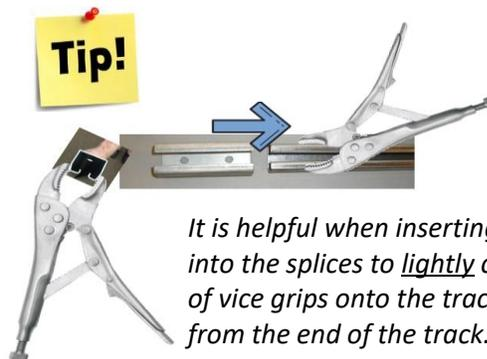
*It is helpful when inserting the track into the splices to lightly clamp a pair of vice grips onto the track about 4" from the end of the track. This narrows the track and allows easy insertion of the splices. Don't pinch too hard or you will deform the track.*
